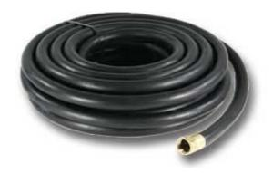
RW1 is general service water hose designed for a wide range of industrial, construction and agricultural applications. It is usually provided as an assembly with brass garden hose couplings thru 3/4", and NPSH pipe thread couplings for 1" and 1-1/2" diameters. RMA class C. -40F to 190F.
